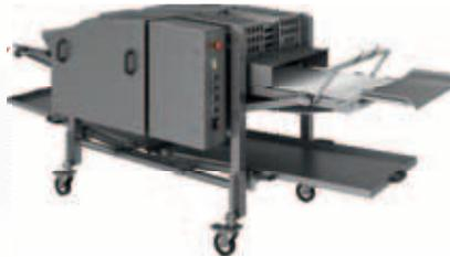
With a Platino in front of a StripCutter, the equal cut strips or dices will be more uniform.
