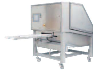
The Marel PortionCutter I-Cut 22 will cut the flattened poultry into more uniform sizes of fixed weight.
